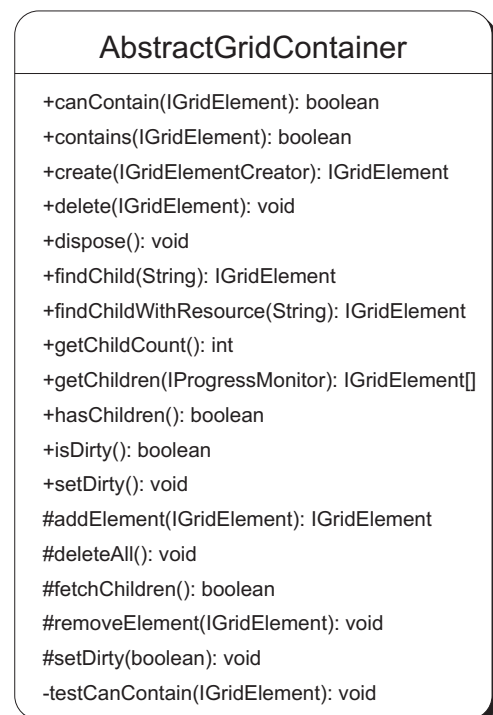
Figure 2.5: The public implementation layer’s AbstractGridContainer and its most important methods.
