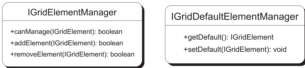
Figure 2.11: The Grid element manager and the default Grid element manager classes and their most important methods in detail.
