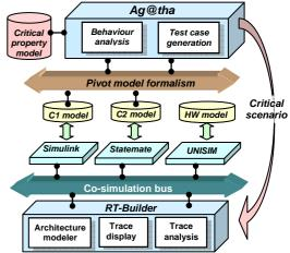
Co-simulation obtained by integrating the various tool simulators in а communication bus with synchronisation protocols and dedicated HMI providing a graphical environment for modelling system architecture, simulating it via the native heterogeneous tool simulators and analyzing monolithic and distributed real time embedded systems.
