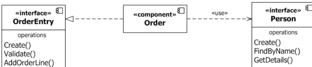
Figure 11.43 Explicit representation of provided and required Interfaces using Dependency notation.
