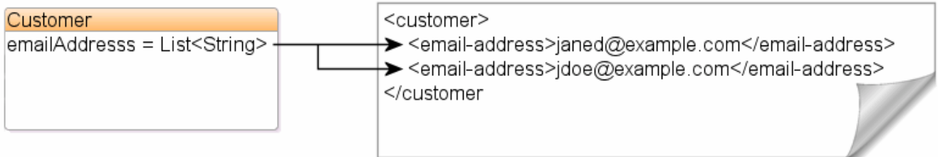
Description of "Figure 4-10 XML Direct Collection Mapping to Text Nodes"
