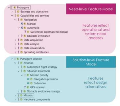
Figure 8: Enrichment of the feature model with architecture alternatives
