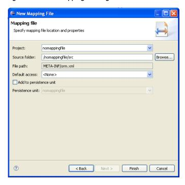
Define the properties in the page and click Finish. The orm.xml file appears in the src directory of the selected JPA project. You can manage the orm.xml file using the JPA Details view or through the XML Editor. See also JPA Details view (for orm.xml).
